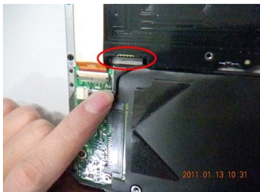
Step 2: Peel off the double sided tape and attach the rubber bumper to the system.
