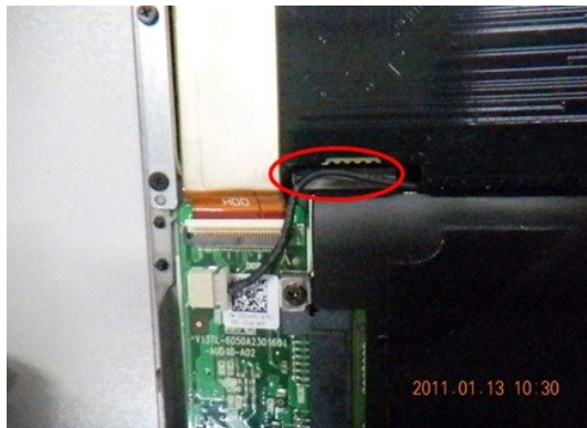
Step 1: Arrange the cable in order to leave assembly space of new rubber.
